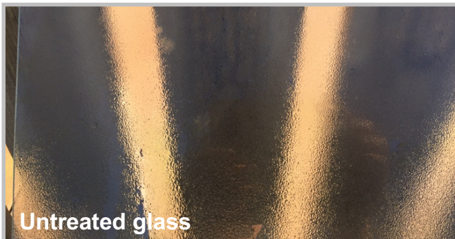
Untreated glass (left) has more condensation droplets compared with glass treated with Prebona Siccol Pro (right).
