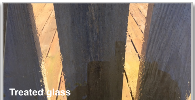
Untreated glass (left) has more condensation droplets compared with glass treated with Prebona Siccol Pro (right).
